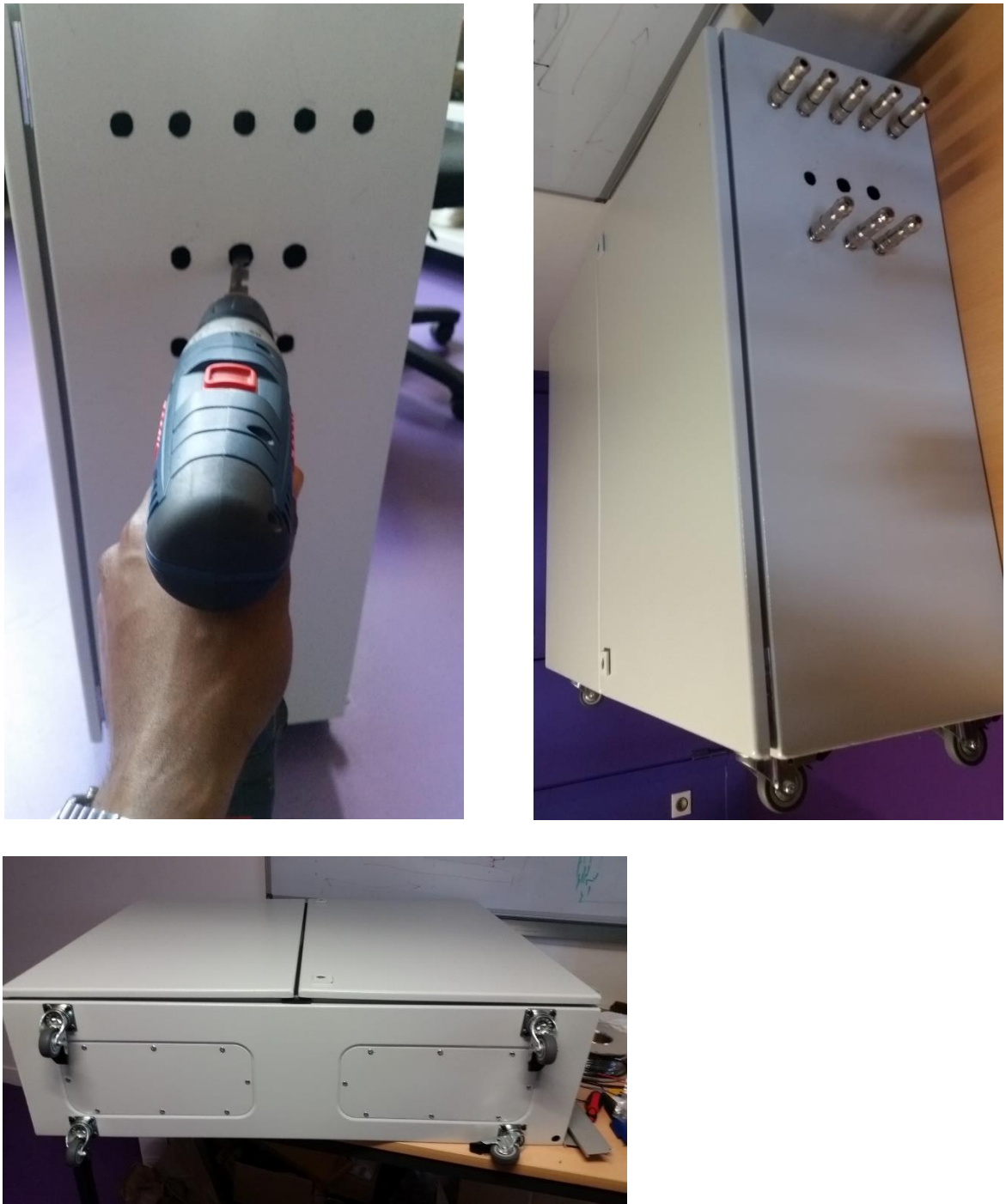
Fig 16: Box drilling holes process
